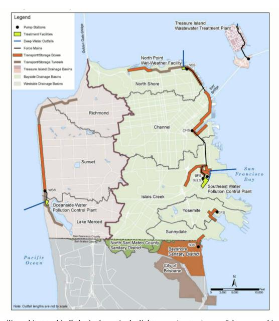
The Facility subject to this Order is shown in the light green (eastern) area of the map and includes the Southeast Water Pollution Control Plant, the North Point Wet Weather Facility, and the Bayside Wet Weather Facilities. The remaining collection system subject to this Order is not shown. The Oceanside Water Pollution Control Plant, Westside Wet Weather Facilities, and Treasure Island Wastewater Treatment Plant are shown only for reference.
